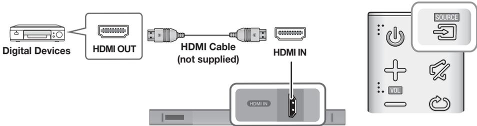
1. Connect an HDMI cable (not supplied) from the **HDMI IN** jack on the bottom of the product to the HDMI OUT jack on your digital device.
